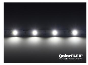
**QolorFLEX LED Tape, Natural White, 12V Indoor (P/N 5050-12-NW-30-5-20-1)** is an interior grade LED tape with a medium output (495 lumens/metre) brightness. The natural white colour (4100°K) equally compliments reds greens and blues. Each LED tape comes with wiring leads on both ends and durable 3M adhesive backing. It is available in full five metre reels and sample strips.
